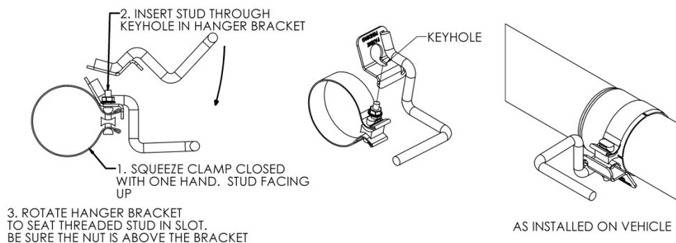
4. Install the front single **Hang Tight™ Hanger Clamp Assembly** (shortest hanger) onto the **4" to 5" Extension Pipe** and into the factory rubber insulator located on the frame.
