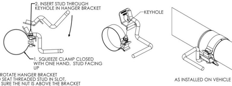
5. Install the **Hang Tight™ Hanger Clamp Assembly** onto the **Extension Pipe** and into the factory isolator. (5.0L shown. On EcoBoost models, use the rear-most factory isolator)
